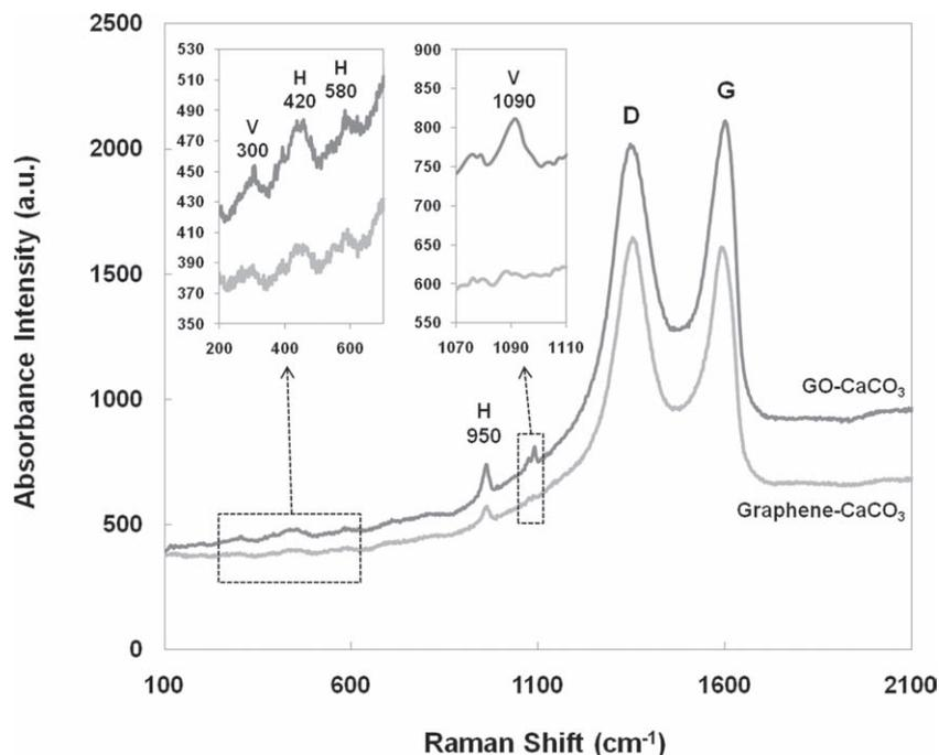
**Figure 4.** Raman spectra of GO/graphene-CaCO<sub>3</sub> hybrid films incubated in SBF for 4 d. Both spectra show characteristic bands at around 420, 580, and 950 cm<sup>-1</sup>, indicating HAP formation. The peak intensities for CaCO<sub>3</sub> vaterite at around 300 and 1090 cm<sup>-1</sup> decreased in the graphene-CaCO<sub>3</sub> hybrid film.
