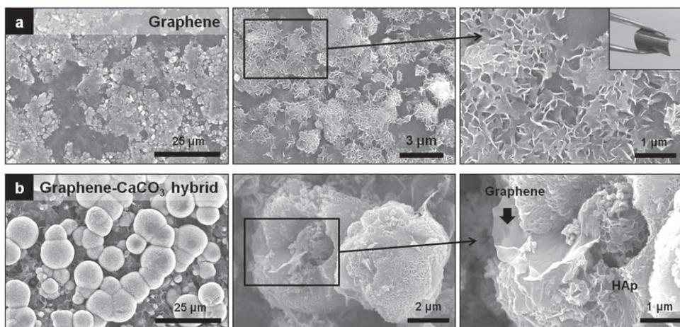
**Figure 3.** A) SEM images of a) bare GO film and b) GO- $\text{CaCO}_3$  hybrid film incubated in SBF for 4 d. B) SEM images of a) bare graphene film and b) graphene- $\text{CaCO}_3$  hybrid film incubated in SBF for 4 d. Both hybrid films hybridized with vaterite (A-b, B-b) showed highly increased formation of lath-like HAp crystals compared to bare GO (A-a) and bare graphene (B-a) films.
