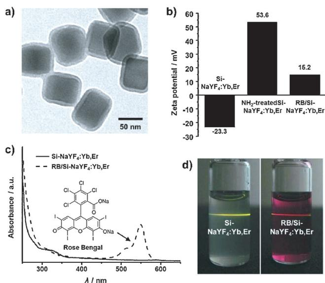
**Figure 3.** a) TEM images of silica-coated NaYF<sub>4</sub>:Yb,Er nanoparticles (Si-NaYF<sub>4</sub>:Yb,Er) dispersed in aqueous solutions. b) Zeta potentials of bare, NH<sub>2</sub>-treated, and RB-bound Si-NaYF<sub>4</sub>:Yb,Er, showing successful binding of RB molecules on the NaYF<sub>4</sub>:Yb,Er nanoparticles. c) Absorption spectra of Si-NaYF<sub>4</sub>:Yb,Er with and without RB. d) Digital camera images of upconversion nanoparticles upon the irradiation of a 980 nm laser.
