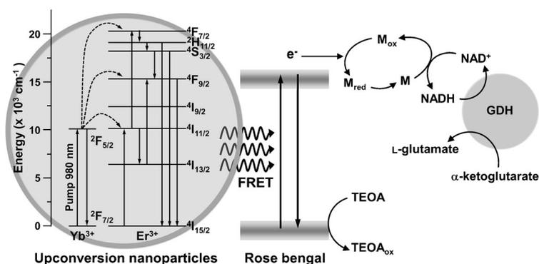
**Figure 1.** Schematic diagram of NIR-light-driven biocatalytic artificial photosynthesis with FRET-conjugated upconversion nanoparticles. The photoexcited electrons generated by RB/Si-NaYF<sub>4</sub>:Yb,Er are transferred to NAD<sup>+</sup> through the rhodium(III)-based mediator (**M**), and then used to synthesize L-glutamate by GDH. TEOA = triethanolamine.
